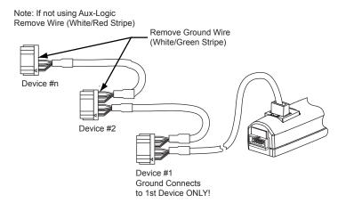
Figure 4.2 Multi-drop communications using the VW3L3D02R30
