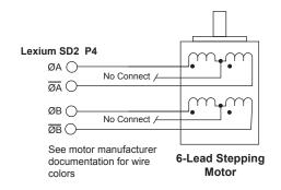
Figure 4.7 6-lead motor full coil configuration
