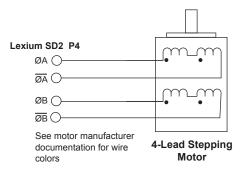
Figure 4.8 4-lead motor connection
