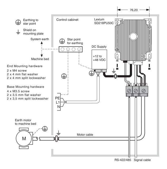
Figure 3.1 Lexium SD218PU50C mounting
