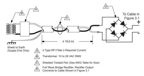
Figure 3.2 15,0 m or greater, AC power to full wave bridge
