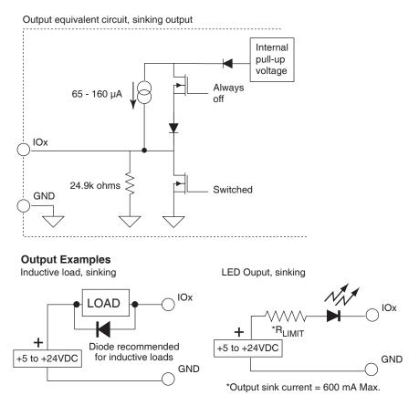
Figure 6.2 Sinking output equivalent circuit and interface examples
