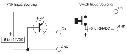
Figure 6.3 Sourcing input equivalent circuit and interface examples
