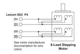
Figure 4.5 8-lead parallel connection
