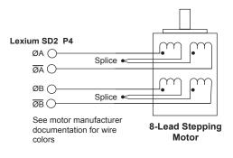
Figure 4.4 8-lead motor series connection
