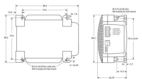
Figure 2.1 Lexium SD218PU50C mechanical specifications
