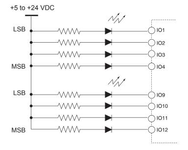
Figure 6.8 Output interface to I/O banks as a group for BCD process control
