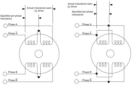
A: 8 lead stepping motor series configuration
