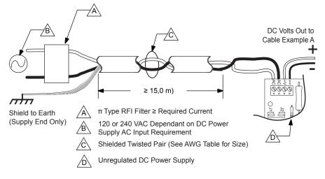
Figure 3.3 15,0 m or greater, AC power to DC supply
