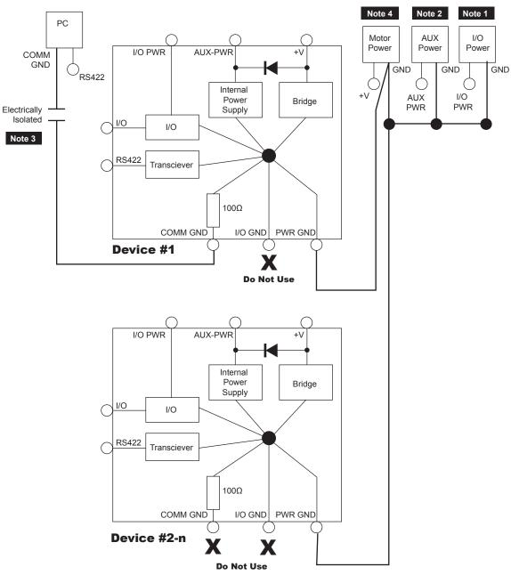
The power connection schematic in Figure 5.7 represents the recommended power configuration for avoiding communications ground loops
