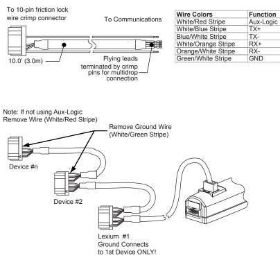
Figure 5.4 Multi-drop communications using the VW3L3D02R30
