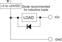
Figure 6.4 Sourcing output equivalent circuit and interface examples
