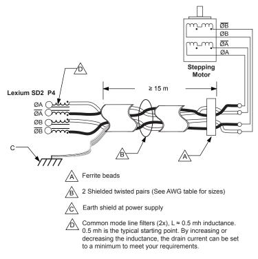
Figure 4.3 Motor cabling over 15,0 m
