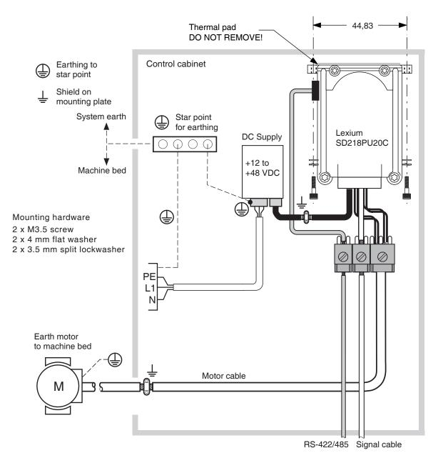
Figure 3.1 Lexium SD218PU20C mounting
