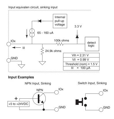
Figure 6.1 Sinking input equivalent circuit and interface examples
