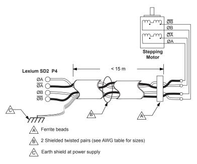
Figure 4.2 Motor cabling under 15,0 m
