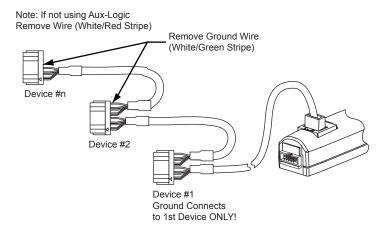
Figure 4.2 Multi-drop communications using the VW3L3D02R30
