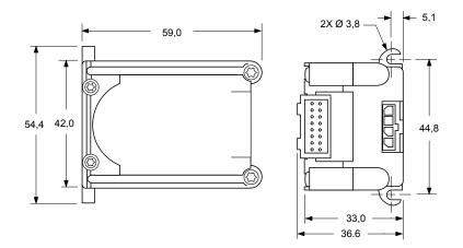
Figure 2.1 Lexium SD218PU20C mechanical specifications
